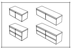
For the UN160W double models. Install both UN080W units on the wall independently, ensuring that they are level. Then install the countertop, securing it to the units with a suitable silicone adhesive.
