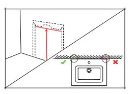
Mark the location of both mounting plates ensuring that they are positioned inside the side panels of the unit. The recommended height for the unit including basin is 850mm.
