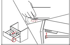
Locate the hangers onto the wall mounting plates.
