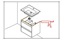
Locate the plates on the inside walls of the unit onto the wall mounting plates. Secure the unit to the wall by tightening the screw. Use a spirit level to ensure the unit is balances horizontally.
